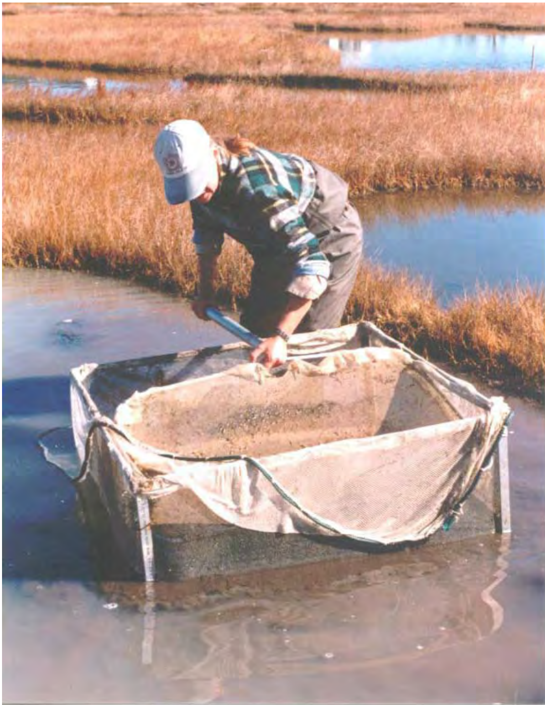
Figure 7. 1m 2 throw trap. The investigator is sweeping the trap with the 1m x 0.5m dip net. Note the skirt of 3mm nylon mesh net attached to the top of the trap for sampling in deeper water.
